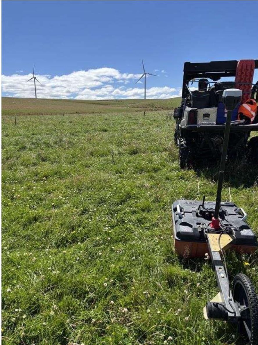
Southern Geophysical conducting a GPR survey on a wind farm site
