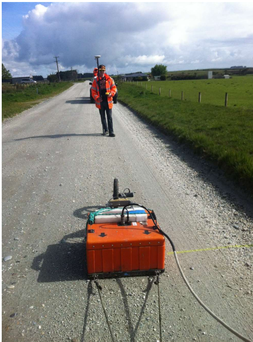
Southern Geophysical conducting a GPR survey
