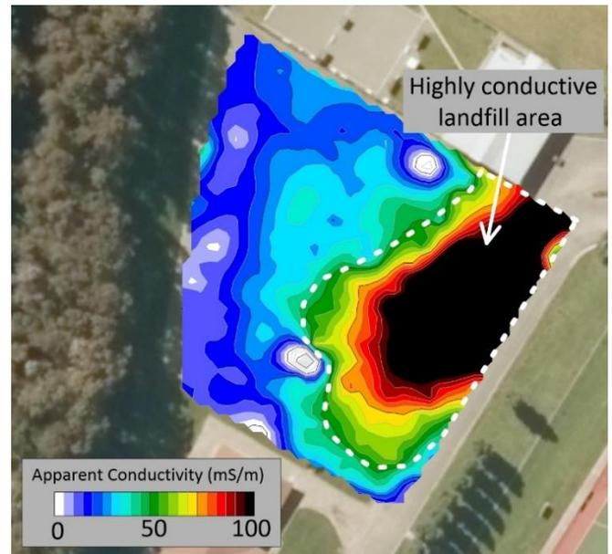
**Below - A GPS synced hypersensitive metal detector (EM61)** can be extremely useful in clearly defining the extents of ferrous metal landfill materials when they are within the upper two metres of the subsurface. With the position of the unit captured in real time, surveying is not only quick but extremely accurate.
